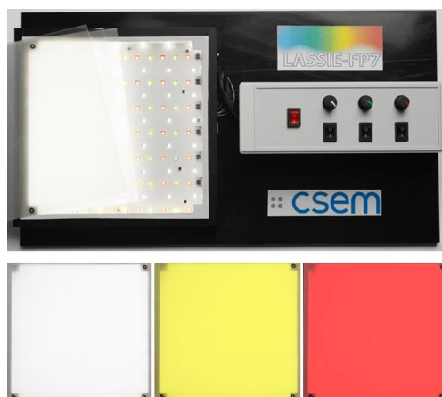
Top) 20x20cm 2 LED-based lighting module with (left) and without (right) a multilayer light management solution developed by CSEM in the European project LASSIE-FP7. The multilayer solution transforms the non-homogeneous light pattern produced by the point-like LED sources into a spatially uniform emitting surface. The module height, 18mm is lower than the LED pitch (30mm). The light engine contains white, red and green LEDs for color tuning. Bottom) Emitting surface of the module tuned to different colours demonstrates that CSEM light management solution offers also excellent light mixing characteristic.
