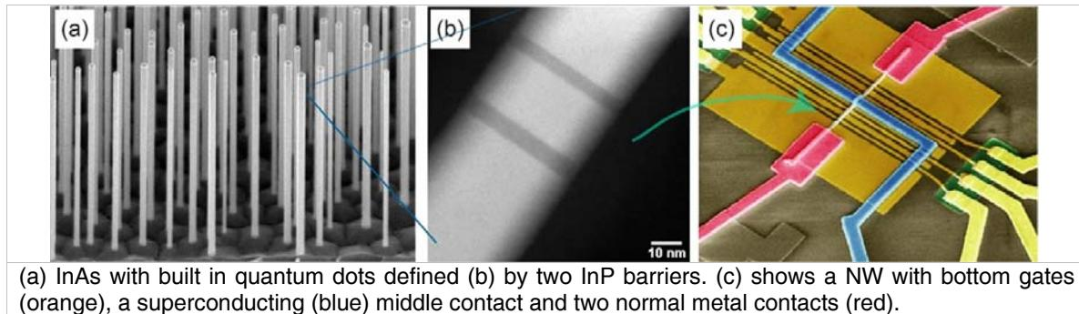
(a) InAs with built in quantum dots defined (b) by two InP barriers. (c) shows a NW with bottom gates (orange), a superconducting (blue) middle contact and two normal metal contacts (red).
